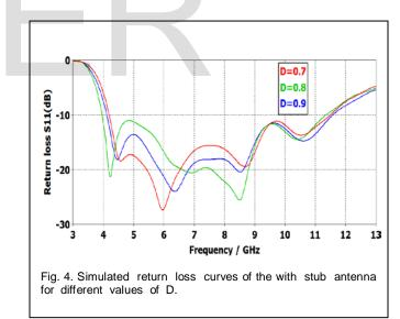
The measured return loss below -10dB.The simulated Return Loss of the with stub antenna achieved by operating frequency (3.9 to 11GHz).In Fig. 4 shows the simulated Return Loss of antenna in the terms of D. Return loss is the parameter which indicates the amount of power that is loss. Return loss is loss of signal power resulting from reflection caused at a discontinuity in transmission line or optical fiber. For D=0.8, 0.7, 0.9 other dimensions fixed It is found that the input
