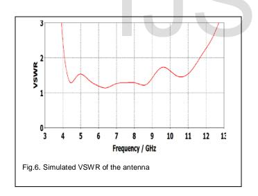
Fig. 6 being evidence of VSWR for beyond the required band width of 3.9 to 11 GHz with (VSWR <2).
