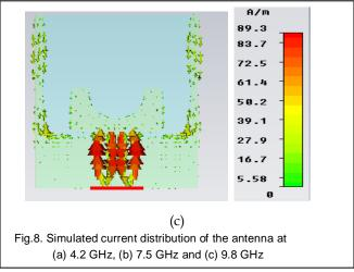
On the other hand, the intermediate and higher frequency resonances are more determined by the elliptically edged small-size radiator, which is able to provide similar current distribution patterns with different, continuously tuned electrical resonance lengths. The surface current distribution compare the frequencies of 4.2, 7.5, and 9.8 GHz. shown in Fig 8 .Shows that the frequency resonance is dominate in increase of current 9.8 GHz.
