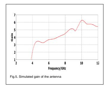
In Fig. 5 presents the simulated gain for antenna. The antenna gain in the UWB band is about 2–6.2 dBi.UWB band frequency range is 3.9 to 11 GHz. It is assumed that the antenna is receiving a signal in the direction of maximum gain. It is also common for the gain to be expressed in decibels and referenced to an isotropic source.
