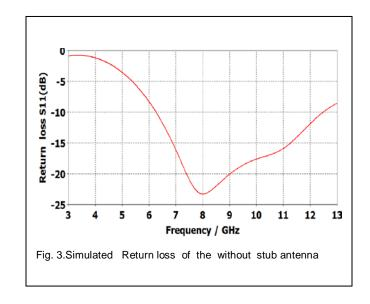
The frequency range from without stub antenna is 6.8 to 10.1 GHz. This frequency range is achieved by return loss value below -10dB.In Fig. 3 simulated Return Loss of the with stub antenna.
